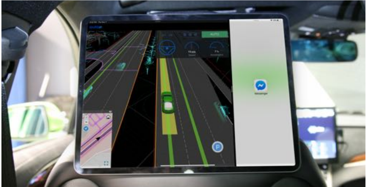
c. touch-screen Human-machine Interface (HMI) console
