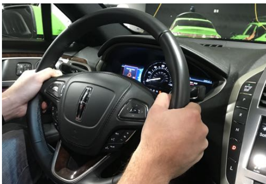
ii. steering takeover: turn the steering wheel for at least one half revolution
