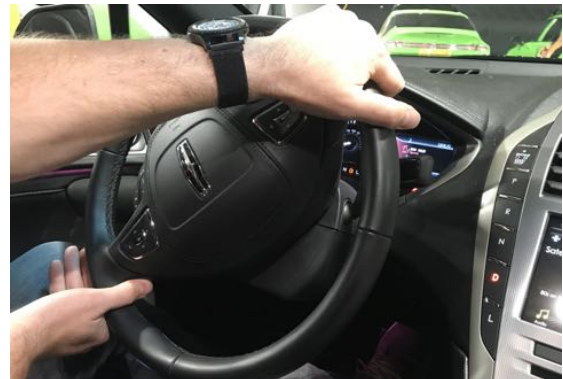
ii. steering takeover: turn the steering wheel for at least one half revolution
