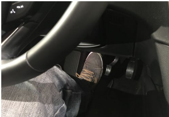
i. brake takeover: press the brake pedal
