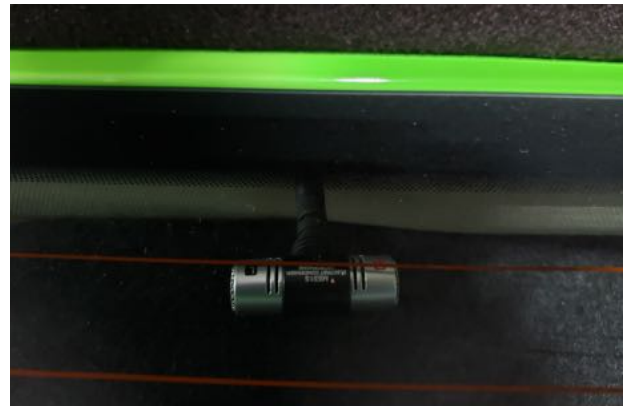
The on-board microphone is capable of detecting and recognizing the siren sounds of emergency vehicles.
