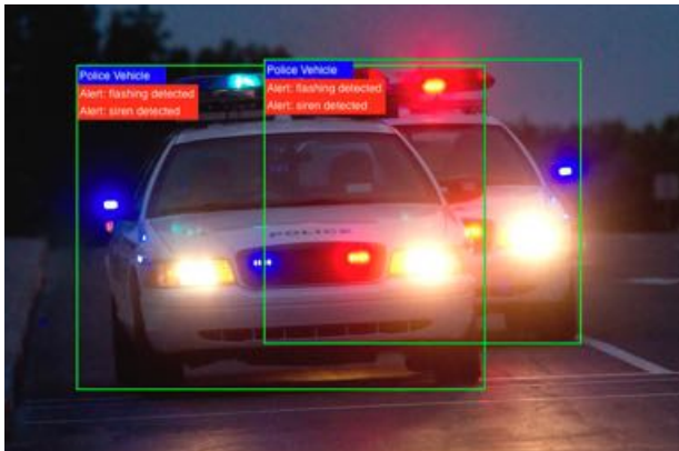
AutoX driverless test vehicle is capable of detecting police and emergency vehicles and performing an automatic pull over.
