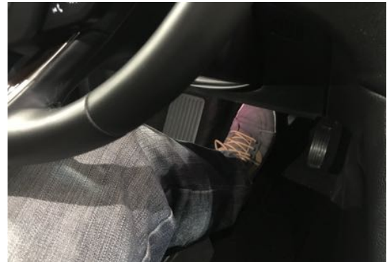
i. brake takeover: press the brake pedal
